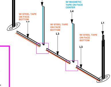
**CENTER POST FOOT** VERTICAL GRAPHIC BAR CENTER POST Make sure to place VERTICAL GRAPHIC BAR with the CENTER POST FOOT facing DOWN
