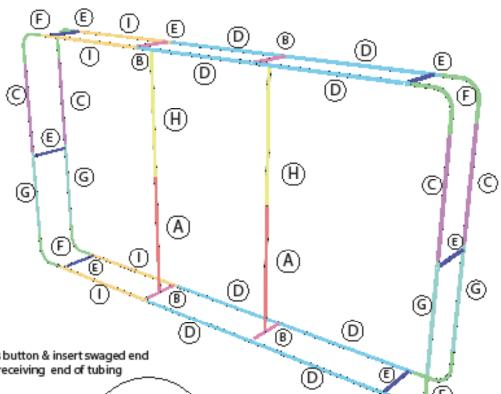
Press button & insert swaged end into receiving end of tubing
