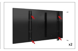
**Step 8: (A)** Hang the monitor onto base plate to test the positioning. Once position is correct remove monitor and add graphic to frame.
