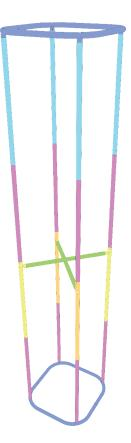
Press button & insert swaged end into receiving end of tubing
