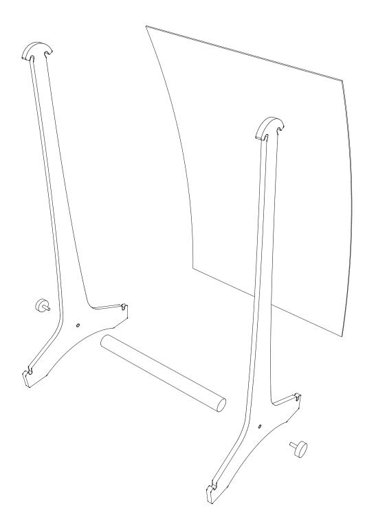
1) First, attach vertical sections to round pole with aluminum caps or bolts.
