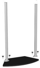
**Step 4**. Attach counter to column using 1 **long** knob. (K0.2 kiosk has counter front & back)
