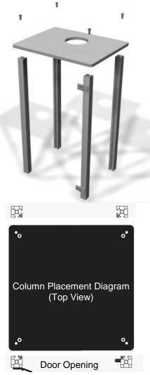
**Step 2**. Attach support column to base using two **short** thumb knobs; install gusset caps.
