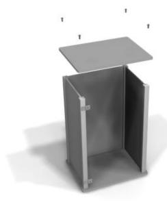
**Step 4.** Attach cabinet door using ½"-20 x ½" button head cap screws. Tighten w/ 5/32" hex key. (**do not over tighten**)
