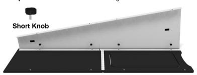
Step 2. Carefully stand up unit. Attach right sides to front using 4 short knobs.
