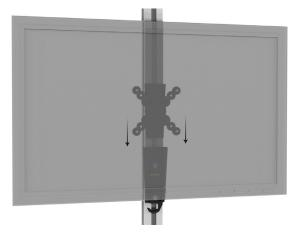
**Step 4.** Slide monitor bracket into mounting plate.
