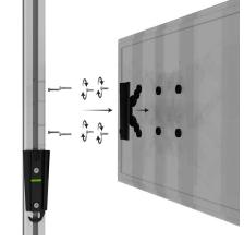
**Step 3.** Attach spacers(if needed). Choose M4 screw set that fits your needs attach monitor bracket to back of TV.
