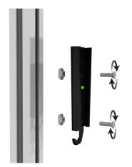
**Step 1.** Insert ×2 1/2" Flathead screws through mout plate; attach s-nuts.
