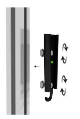
**Step 2.** Insert s-nuts into XV extrusion channel.
