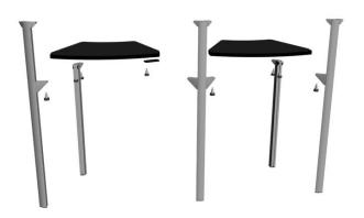
**Step 2**. Attach transaction tops & joining plate. (there are 2 holes at termination end)
