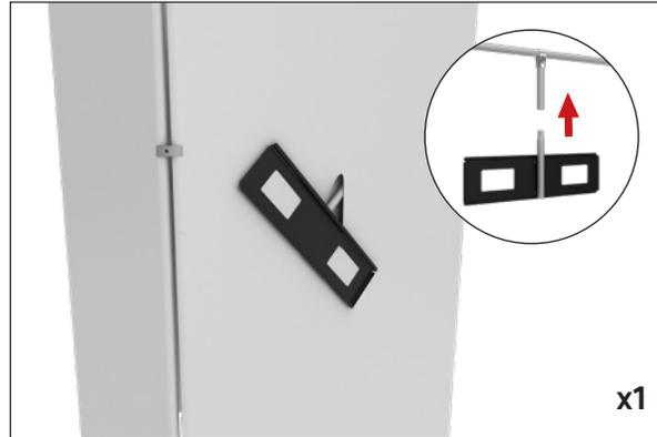
**Step 7:** Attach brackets to back of monitor with screws. Rubber spacers can be placed between the bracket and the monitor if your the back of the monitor is not flat. Choose the spacer that best fits your need. Position the VESA bracket with the **hook facing down.**
