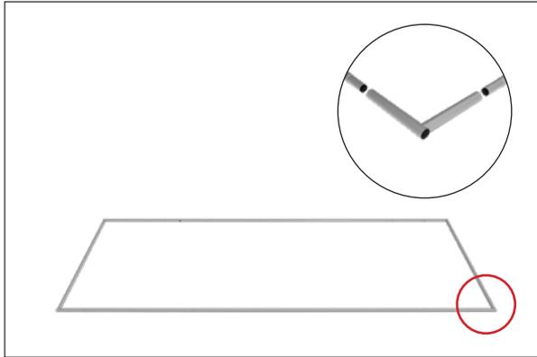
**Step 2:** Connect crossbar to frame using hex bolt and tool.
