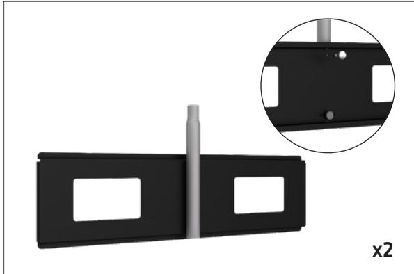
**Step 8:** Insert the Vesa Plate Bracket with bottom pole into the fabric opening and click into top hanging pole. **Important - make sure button is clicked into pole and secure.**
