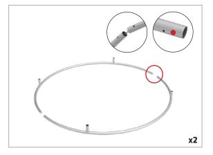
**Step 4:** Slide graphic over frame and zip closed at bottom. **Important! Line up holes in top of frame with holes in graphic.**
