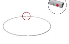
**Step 12:** Unzip print and place one frame inside. Position holes on frame to align with eyelets in graphic. Thread cable through eyelet. Repeat for all eyelets.
