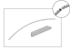
**Step 11:** Align top frame to bottom frame and push support poles into the frame. With some force connect the support poles in the middle to complete.
