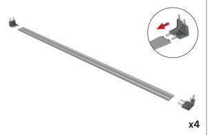
**Step 4:** Build the center support pole by push sections together.
