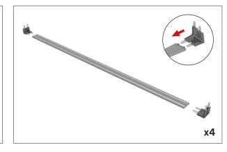
**Step 4:** Join the 2 vertical side frames to top and bottom horizontal frames.
