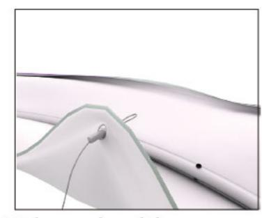
6.Thread cable support through eyelet.
