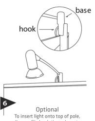
align profile hook through center groove of light base.
