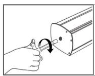
Insert re-tension tool into the right side opening. Holding tool firmly, twist 33 full turns clock-wise to re-tension.
