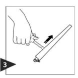
Remove endcaps off the profile bar. Use the edge of Re-Tension Tool to open the snap-lock profile.
