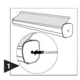
Pull graphic out until the leader is exposed. Insert locking pin to disable the roller.
