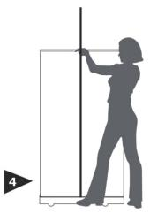
Pull graphic out of base and fasten hook into top of pole.
