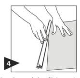
Once the snap-lock profile is open, insert top portion of graphic into profile.
