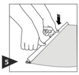
Apply even pressure to the snap-lock profile to lock graphic into place.
