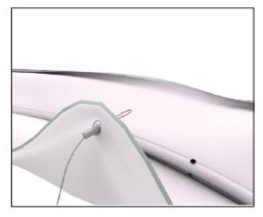
6.Thread cable support 7. Place the black through eyelet.
