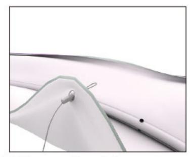
6.Thread cable support through eyelet.
