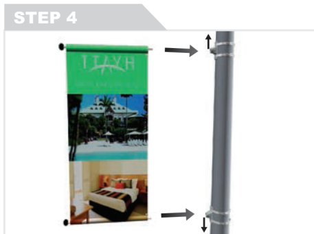
STEP 4 Insert poles into holes on bracket (bracket position may need adjustment)
