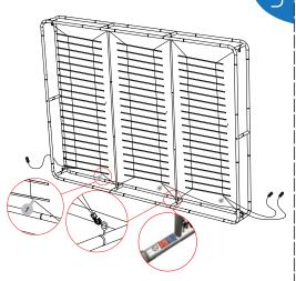
Hang the LED lights into the frame sequentially, paying attention to the direction of the LED panel (see page 1)
