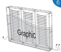
Pull the graphic onto the frame from the bottom up. For single-sided displays the lights should face AWAY from the image. (The power cords for the lights should be pulled out from the holes in graphic)
