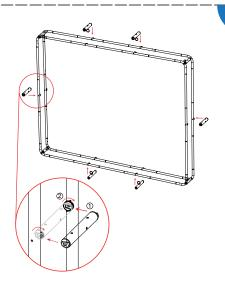
Install the rest of the horizontal support connectors
