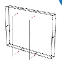
Install the vertical support tubes to finish the frame
