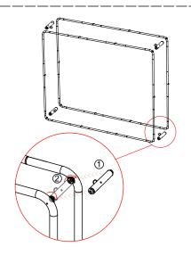
Install the four corner horizontal support tubes first.
