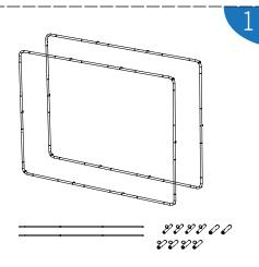
Put together the front and back large tube frames, as the picture shown, and prepare the center support tubes
