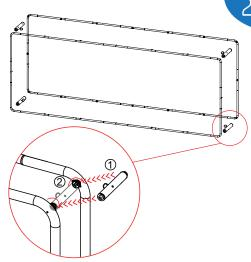
Install the four corner horizontal support tubes first.
