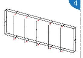
Install the vertical support tubes to finish the frame
