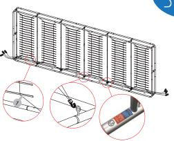
Hang the LED lights into the frame sequentially, paying attention to the direction of the LED panel (see page 1)
