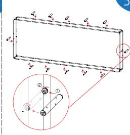
Install the rest of the horizontal support connectors
