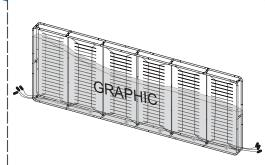
Pull the graphic onto the frame from the bottom up. For single-sided displays the lights should face AWAY from the image. (The power cords for the lights should be pulled out from the holes in graphic)
