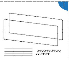
Put together the front and back large tube frames, as the picture shown, and prepare the center support tubes
