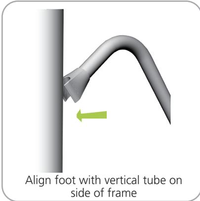
Align foot with vertical tube on side of frame
