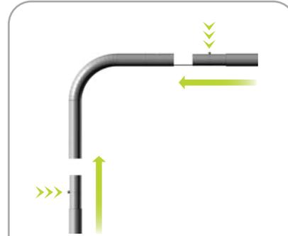
Connect corners of frame by lining up holes with snap buttons
