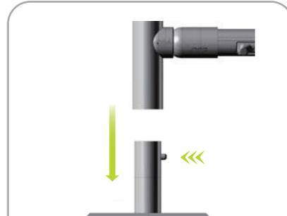
Connect frame to feet by lining up holes with snap button on feet
