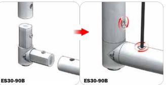
Compress one unlocked end of the connector and slide it through one tube end. Compress the other end of the connector and slide the second tube on. Lock both screws carefully using your hex key tool. Be sure to lock securely, but do not overtighten.
