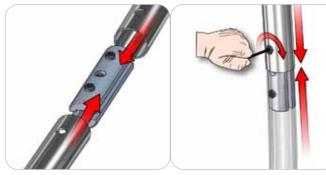
Compress the unlocked connector and slide one tube onto each end. Lock both screws carefully using your hex key tool. Be sure to lock securely, but do not overtighten.
