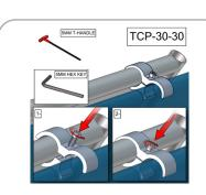
Using provided 5mm hex key, rotate bolt clockwise to secure accent to top of fabric backwall.
