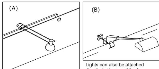
Lights may be attached to top of units with headers by using a standard Nimlink clip into the PT header rail. (A)
