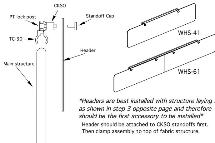
*\*Headers are best installed with structure laying flat as shown in step 3 opposite page and therefore should be the first accessory to be installed\**
