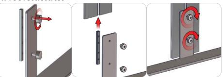
First, loosen the thumb screws and channel bars on the stabilizing bases. Do not disassemble them. Second, slide channel bars into the frame channel flush with the base of the frame. Third, tighten the thumb screws and channel bars securing the attachment. Do not over tighten the thumb screws.
