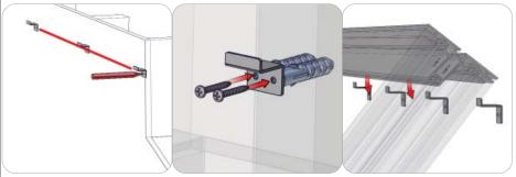
First, find the wall studs and mark a leveled horizontal line. Second, us the provided screw hardware to fasten the bracket into the wall studs. Fasten the brackets on center of each stud for maximum strength. Third, place the assembled frame with graphics and opaque liner onto the wall mounted brackets. You may have to make cuts to the opaque liner to access the frames internal channels, if pre-assembled cuts are not provided. (tools not included for this step)
