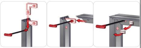
First, insert the corner connector into the extrusion while holding in the lock button with the allen key tool. Second, slide the next extrusion onto the same corner connector while holding in the lock button using the allen key tool. Third, use the allen key tool for locking the corner connector buttons in place. Use the allen key tool to make half turns clock-wise. Do not over tighten the lock buttons.
