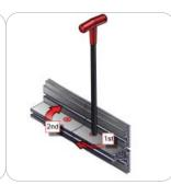
First, insert the in-line connector into the extrusion while holding in the lock button with the allen key tool. Second, slide the next extrusion onto the same in-line connector while holding in the lock button using the allen key tool. Third, use the allen key tool for locking the in-line connector buttons in place. Use the allen key tool to make half turns clock-wise. Do not over tighten the lock buttons.
