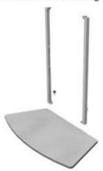
Step 2. Attach v-legs to counter top using two long knobs.
