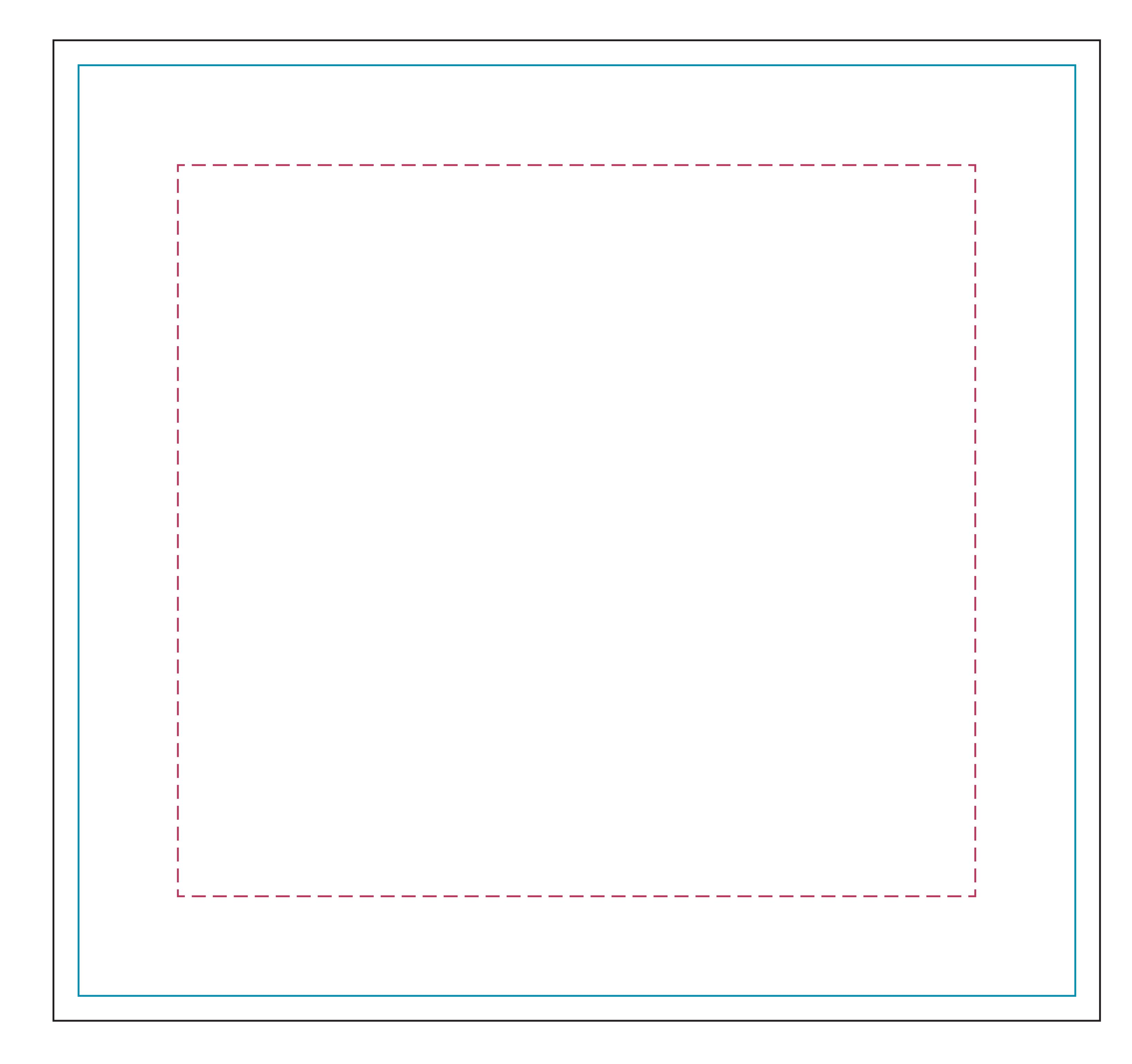
X-FACTOR: A term describing the result of tension at all corners and connection points of an Xpressions skin when placed on a frame. The artwork will be stretched with the least amount of distortion at the center of each quad, and the most distortion within the outer 3-5" of the skin. It is not a live area, as the image will be visible.
