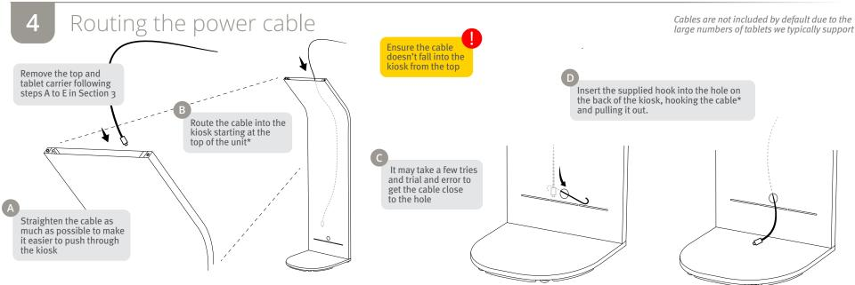
Cable options differ and although we suggest routing from the top of the kiosk – some cables will require routing from the bottom > up due to their design and size.
