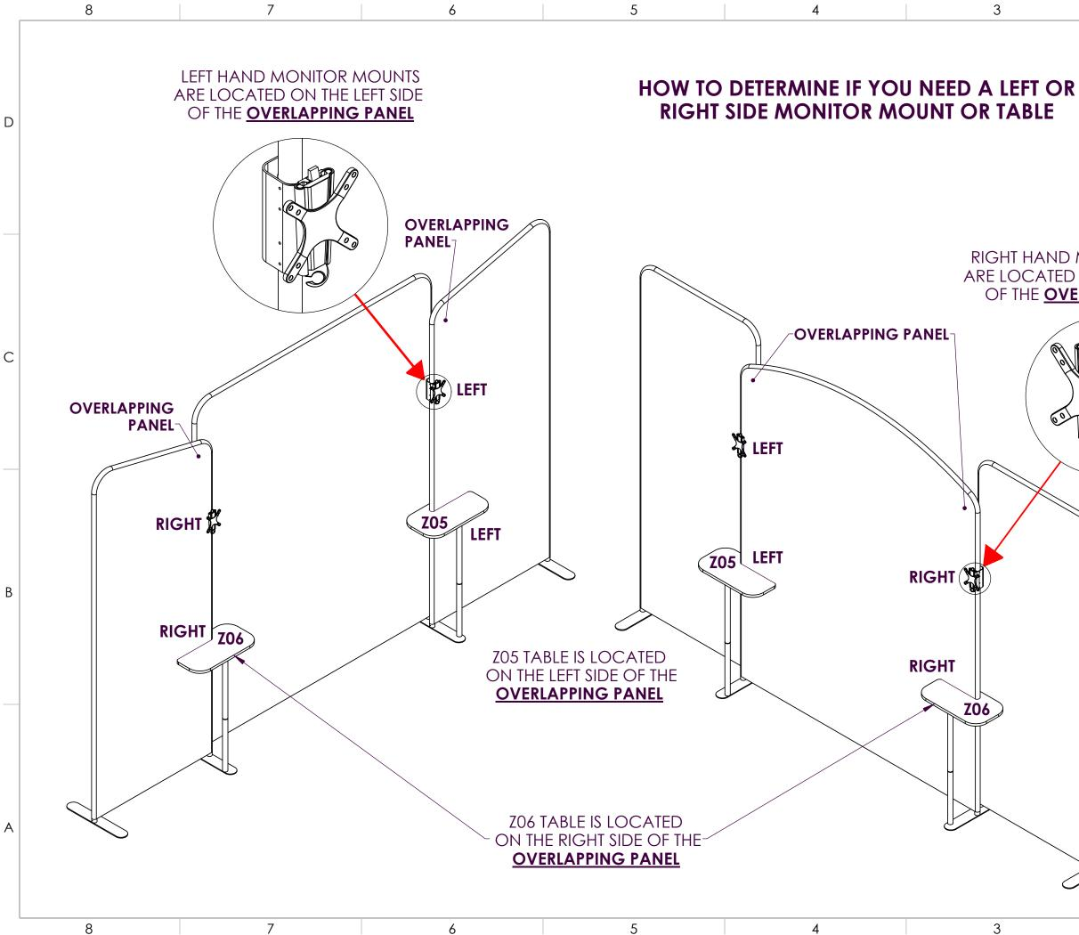
D **RIGHT HAND MONITOR MOUNTS** ARE LOCATED ON THE RIGHT SIDE OF THE **OVERLAPPING PANEL** С В ⊕⊕ THRD ANGLE NIEDO GROUP, INC. 5465 SW WESTERN AVE BEAVERTON, OR 97005 DIMENSIONS ARE IN MILLIMETERS TOLERANCE WAVE TUBE MODULAR MONITOR MOUNT & TABLE DETAIL ENSEMBLE, ASSEMBLY 03 B
