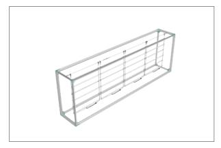
**Step 8:** Fit PVC inner boards onto the top of frame with wedge side face down. Position and align boards until they are all fitted into the frame.
