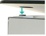
**b.** Place the countertop on top of the counter by aligning the dovetails to the circular caps.
