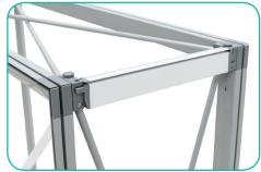
**c.** Attach the top and bottom endcaps on each side of the frame.
