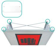
**a.** Locate the circular caps on top of the counter and locate the dovetails underneath the countertop.
